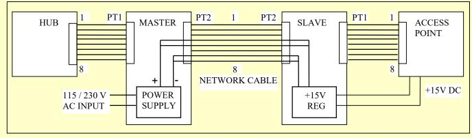
**Warning:** - It is important to be sure that wiring is correct before powering up. Wrong wiring may blow the output fuse in the Master or damage the AP110 or Hub. Contact SMET Ltd for details of the 'CONNECT TEST', a simple network cable tester with visual indication of open and short circuit, sequence, and rotation from pin 1.
